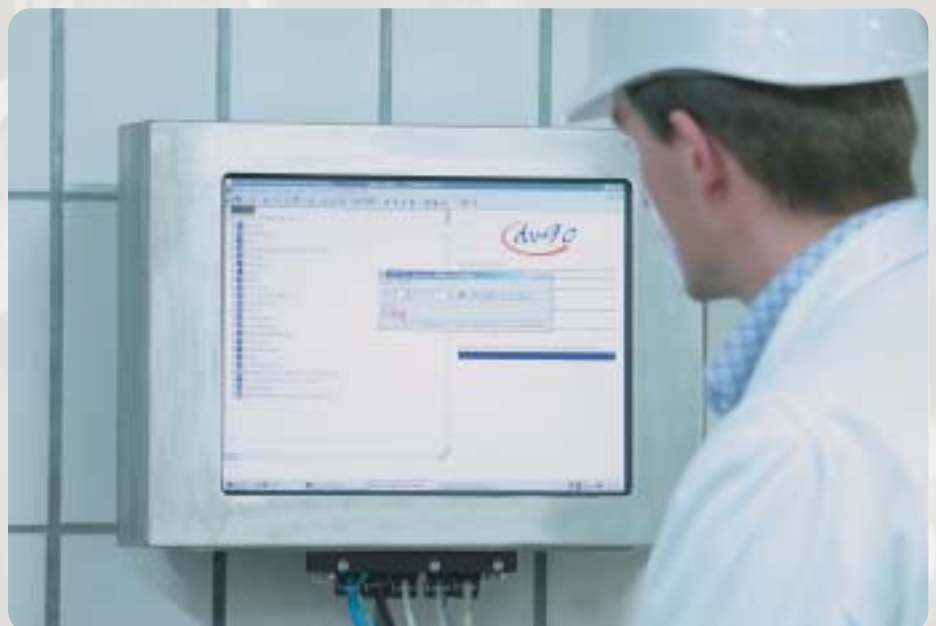
IPC in interaction with Windows-based DV90 QA-software and peripheral devices
