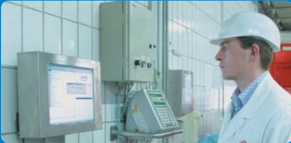
QA at goods outlet: noax S15 IPC in interaction with weighing machine and DV90 QA-software
